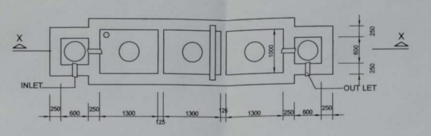
DETAIL PLAN OF SEPTIC TANK FOR 40 USERS SCALE :- 1:50
